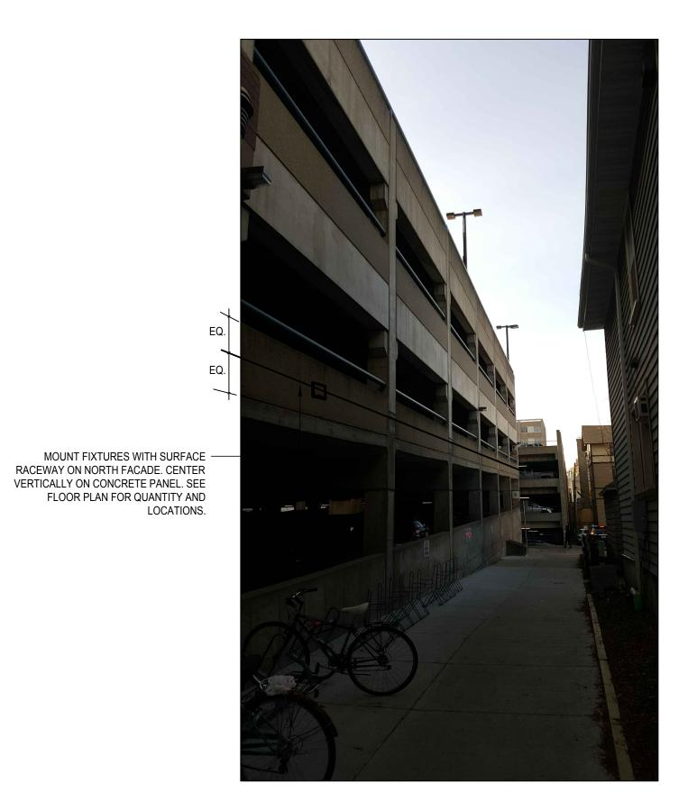
NORTH FACADE LIGHT FIXTURE MOUNTING ELEVATION
